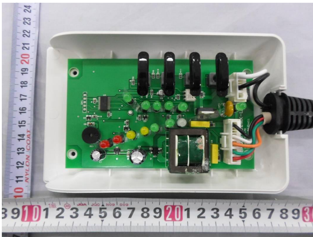
Photo 5 – Internal View of Control box #1
